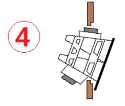
At this moment, the top driver of DDQ has got into the cabinet as you push the top part of DDQ into the cabinet.
