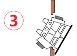
At this moment the bottom part of DDQ has fully got into the cabinet. Next, decrease the leaning angle and try to push DDQ's top part gently into the cabinet.
