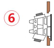
Adjust DDQ and put it into right position. Push DDQ's panel upward from its bottom so that the whole panel gets into the counterbore exactly.
