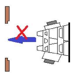
traditional "push in and pull out" method is futile(again the reason is that the height of the main part is greater than its panel. See left picture) and we need a simple trick to install it.
