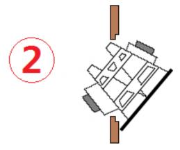
Then **push** DDQ **down** gently so that the bottom edge of the woofer hole in the cabinet goes into the **space** between the DDQ's bottom driver and DDQ's panel. And with the help of gravity the bottom part of DDQ gets into the cabinet.
