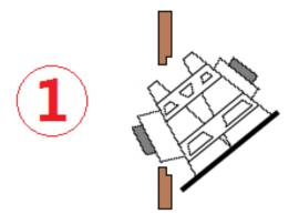
First, make DDQ lean forward. Let the bottom driver(the bottom 'grey' part in the pic 1) go through the woofer hole first.
